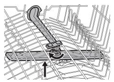
**3.** Wash the spray arm under running water. Use a thin pointed tool, e.g. toothpick, to remove particles of soil from the holes.
