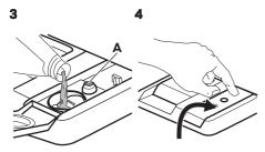
Fill the rinse aid dispenser until the rinse aid reaches the marking "MAX". Remove the spilled rinse aid with an absorbent cloth to prevent too much foam. Fill the rinse aid dispenser when the indicator (A) becomes clear and the rinse aid indicator on the control panel is on.
