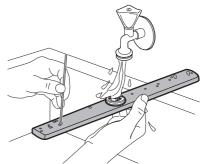
4. To engage again the spray arm to the basket, press the spray arm upwards in the direction indicated by the lower arrow and simultaneously turn it counterclockwise until it locks into place.
