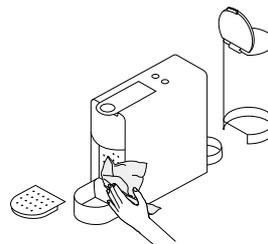
**2 Dry with a fresh and clean towel,** cloth or paper and reassemble all parts. Clean the coffee outlet and inside the machine regularly with a damp cloth.
