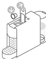
**2** **Lift the lever** completely and insert the capsule.
